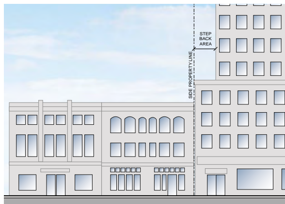
Context-sensitive design integrates new buildings with older ones by stepping down to meet older building heights.
